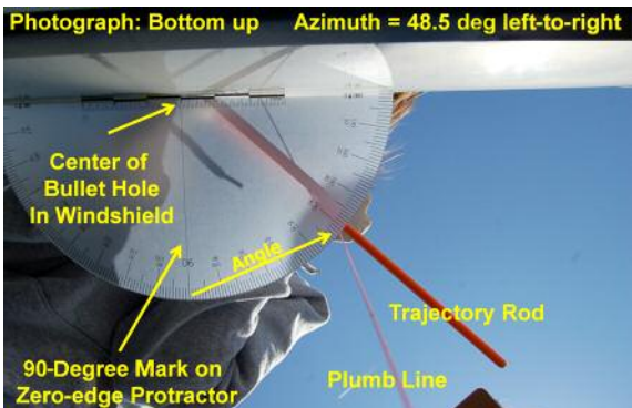
Figure 11.3: Determining the Azimuth Using a Zero-edge Protractor
