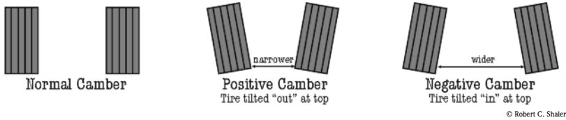
Figure 4.3: Camber Affecting Track Width
