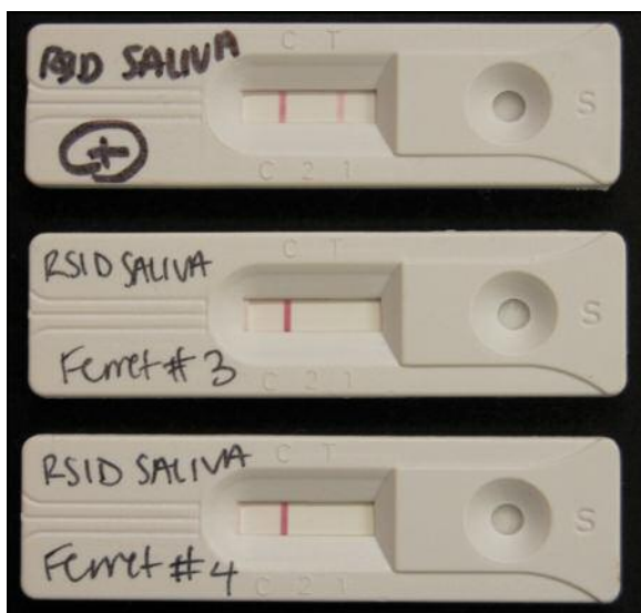
Figure 7.2: RSID Chromatographic Card for Saliva
