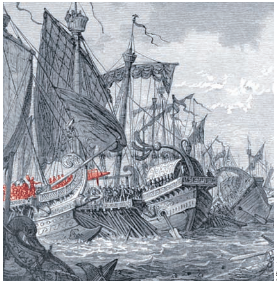
A corvus on the Roman ship in the foreground with Roman Marines lined up prepared to use it (highlighted), attacks a Carthaginian ship during the Punic Wars.
